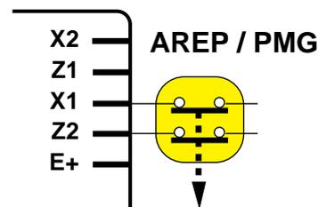
The exciter is switched off by disconnecting the AVR power supply (1 wire on each auxiliary winding) – contact rating 16 A - 250V A.C.
